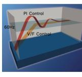
The PI Control is used to control the oil level, temperature and pressure of plant and process. This drive speed control fucntion compares between drive setting value and signal values guaged from sensors and actual contol is made through Proportion and Integral.
