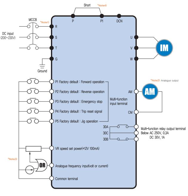
\*Note1) \*• "and "O" means the main circuit and the control circuit respectably. Please connect to the R and S terminals in case of single phase use. .\*Note2) The analogue output is from zero to 10V.
